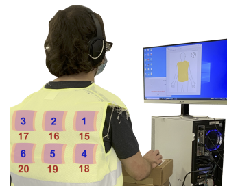
Fig. 3. Experimental setup showing a participant wearing one of the soft haptic vests and interacting with the graphical user interface. Participants could not see the haptic stimuli applied to their back and wore noise-cancelling headphones playing white noise to mask any auditory cues.
