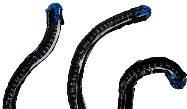
Fig. 1. Photos showing various final robot configurations possible with our proposed shape locking design.
